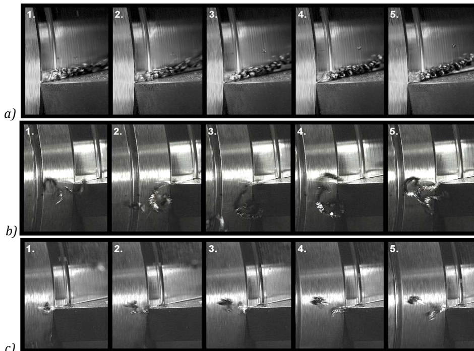
Fig. 14. Influence of feed rate on chip formation (NC10; 62 HRC; a_p=0.3 mm, v_c=120 m/min): a) f=0.058 mm/rev, b) f=0.105 mm/rev, c) f=0.153 mm/rev
